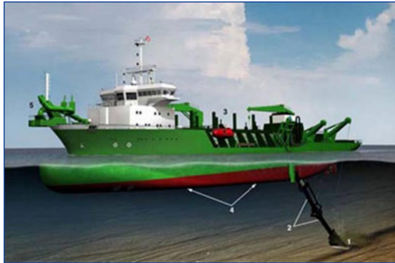
Figure 30: Typical Sub-Sea Pipeline Equipment – Trailer Suction Hopper Dredger
