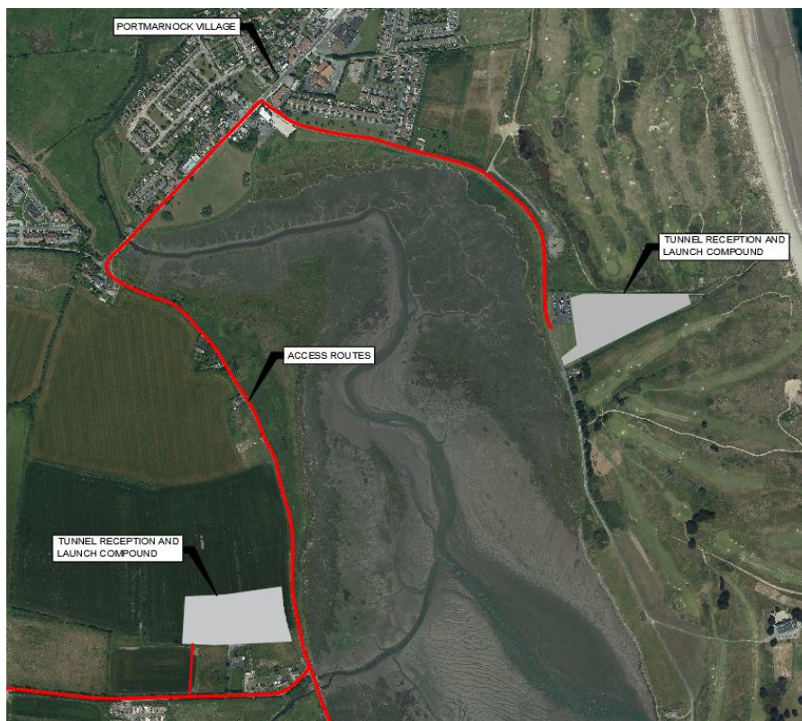
Figure 20: Tunnel Compound Locations
