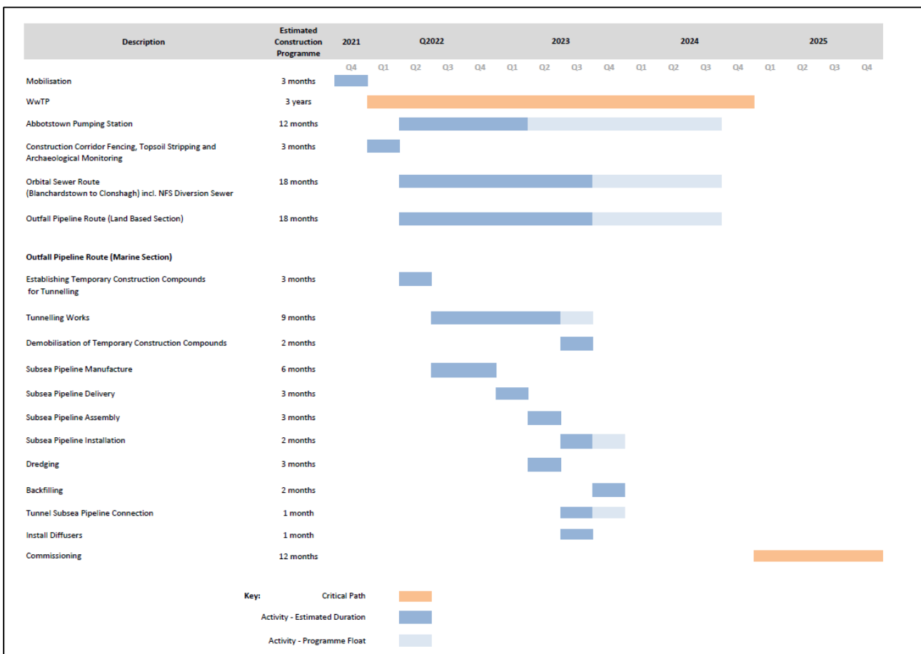
Figure 2: Outline Construction Programme for Orbital Sewer, Abbotstown Pumping Station, WwTP & Outfall Pipeline
