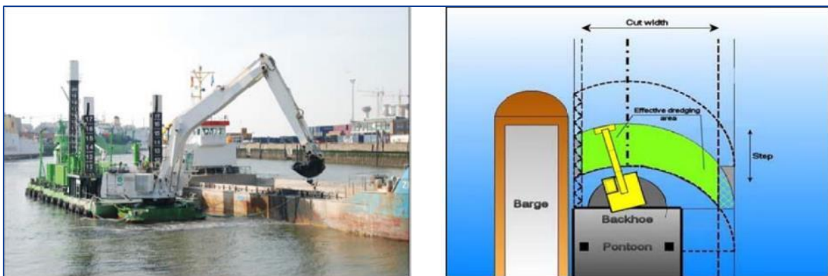
Figure 29: Typical Sub-Sea Pipeline Equipment – Backhoe Dredger
