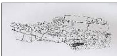
Underwater elevation of bridge pier collapsed in 1763. River Nore Flood Alleviation Scheme
