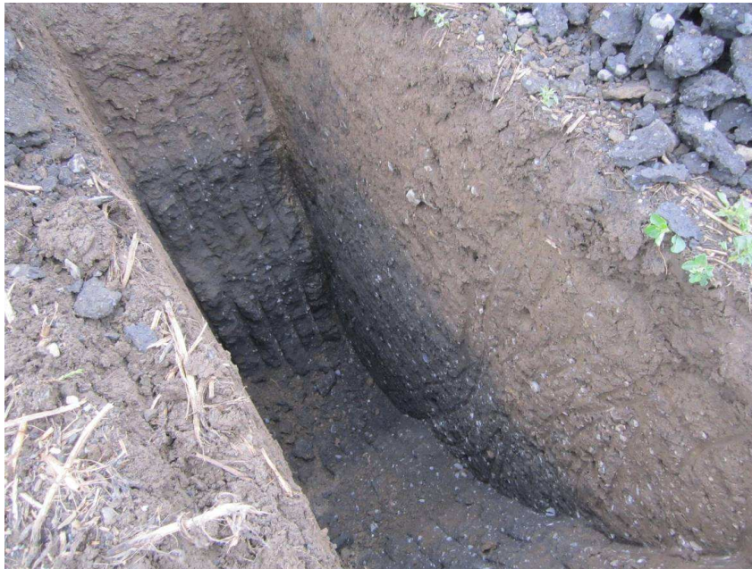
Plate 1 – Typical clay succession observed across the site (exposed in Trial Pit TP16)
