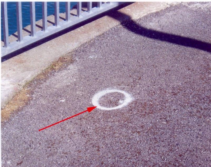
Figure 13. Metal pin in the ground on the pier in Howth Harbour. The RTK surveys carried out by the Marine Institute places this point 3.395m above the Datum at Malin Head.
