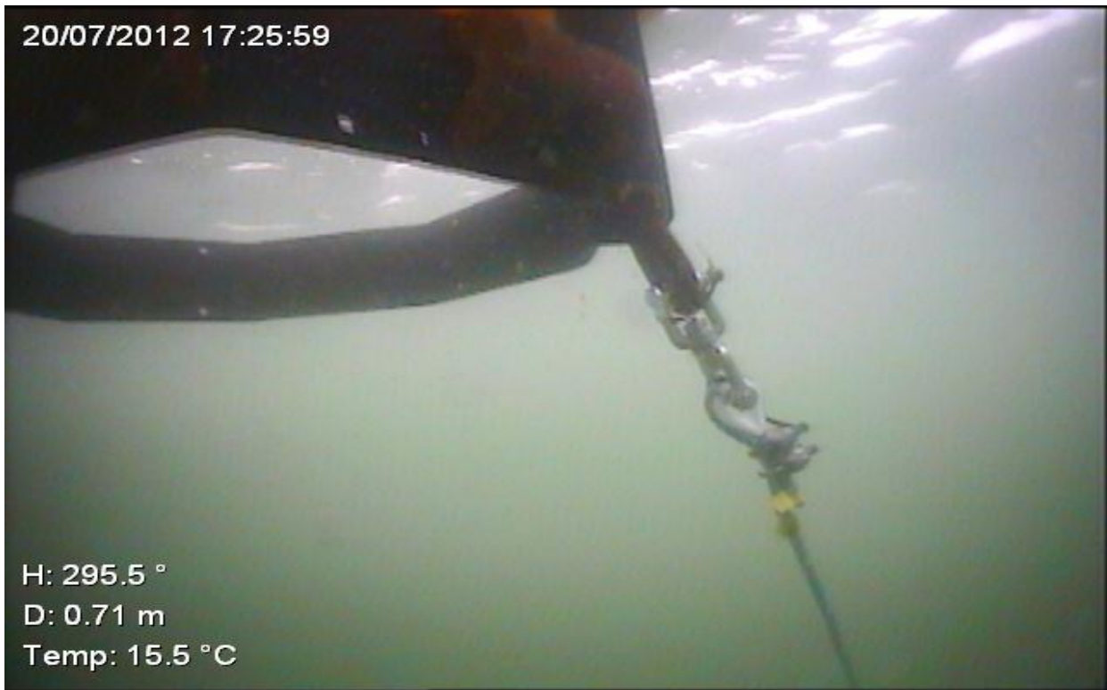
Figure 9. Underside of the marker buoy with swivel shackle connected to mooring cable
