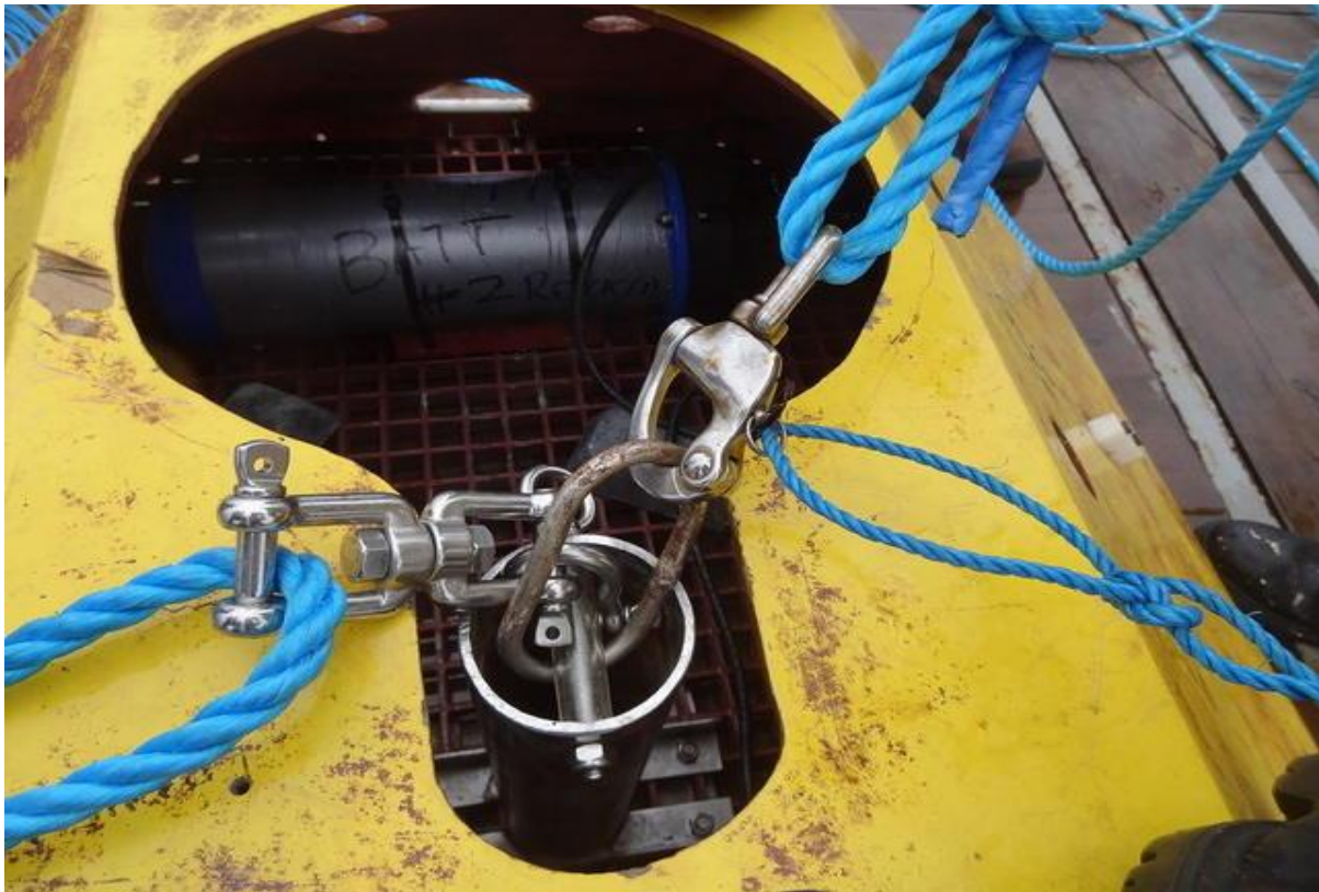
Figure 7. Quick release shackle attached to vertical steel pole.
