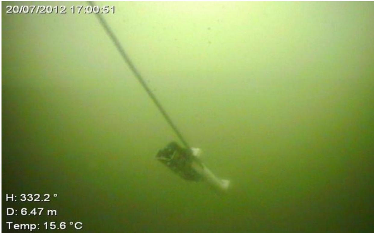
Figure 10. SBE 37 MicroCAT moored on the jacketed combination wire at 7.5m
