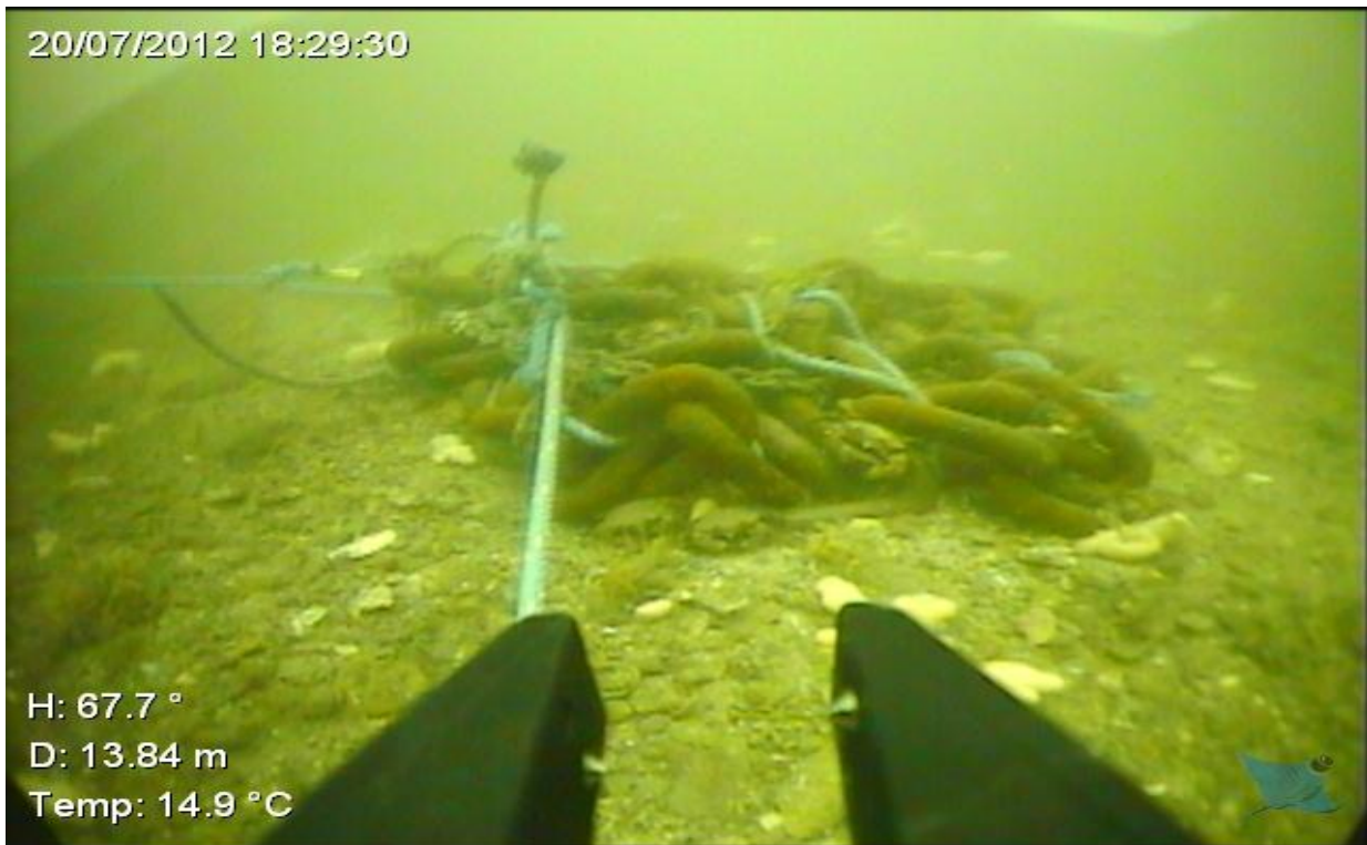
Figure 11. Anchor chain on the seabed at 14m. The two mooring lines coming off the sinker chain lead to the buoy and the AWAC frame.
