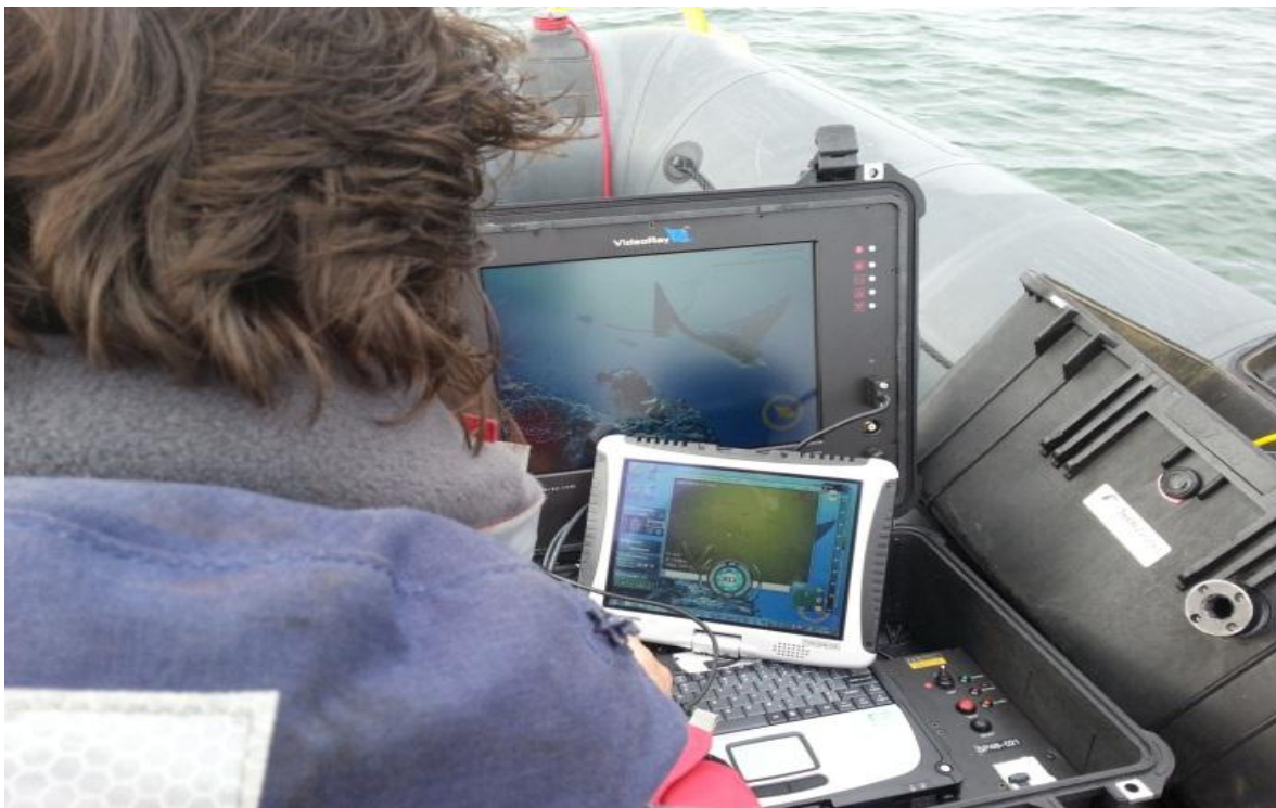
Figure 8. Deploying the ROV from the boat. The deck console is shown which along with the laptop used for recording the video stream to file.
