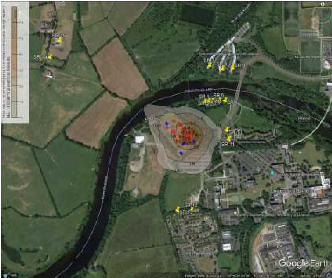
Figure 7-4: Proposed Development to Castletroy WwTP - Predicted Worst-Case 98th Percentile of Hourly Average Odour Concentrations 2021.
