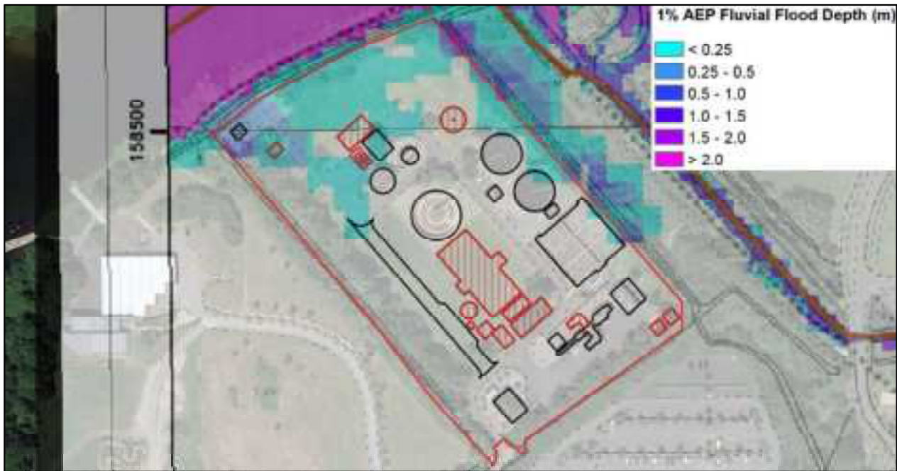
Figure 14-12: Flood Depth Map (1% AEP) with Proposed Infrastructure
