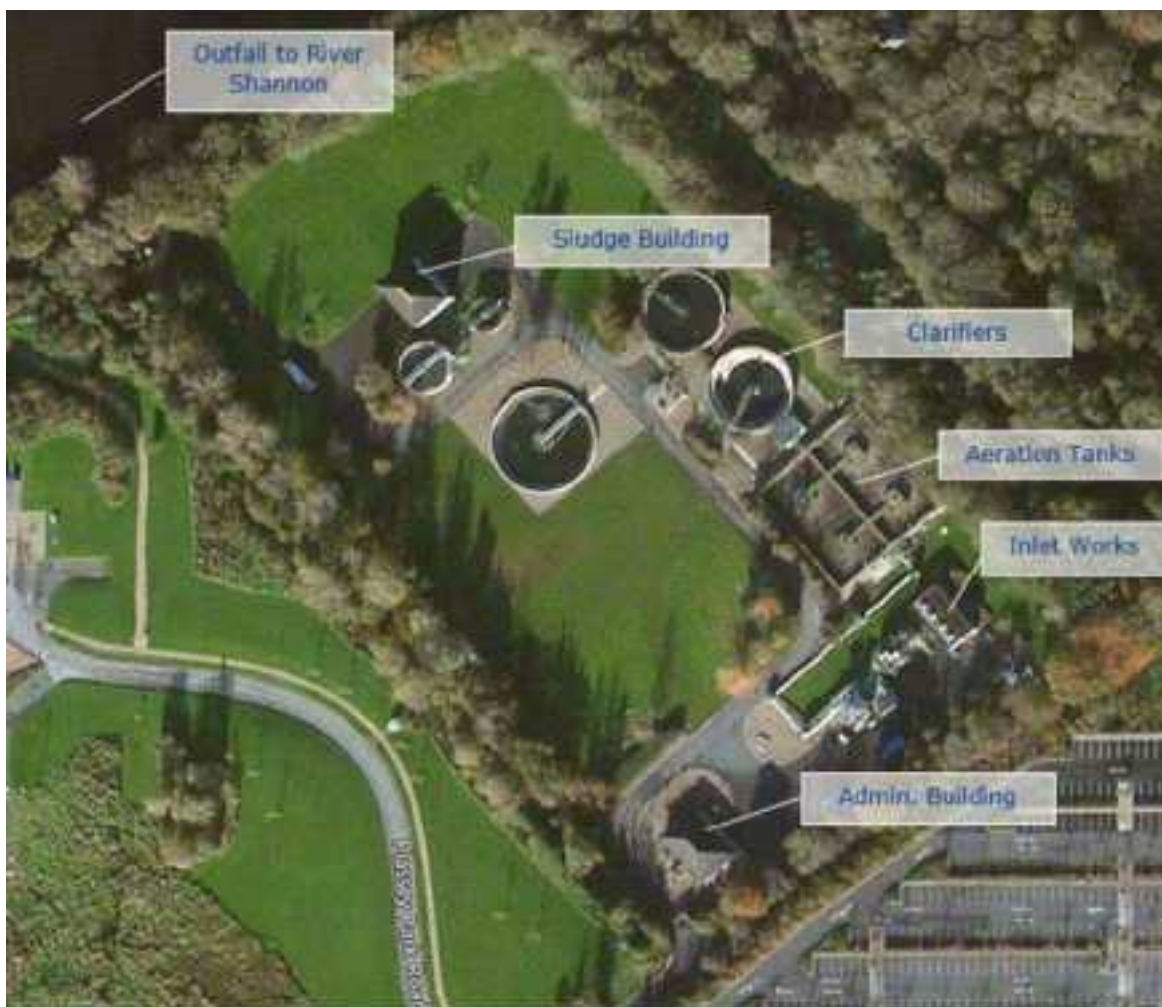
Figure 1.3: Castletroy WwTP Existing Layout
