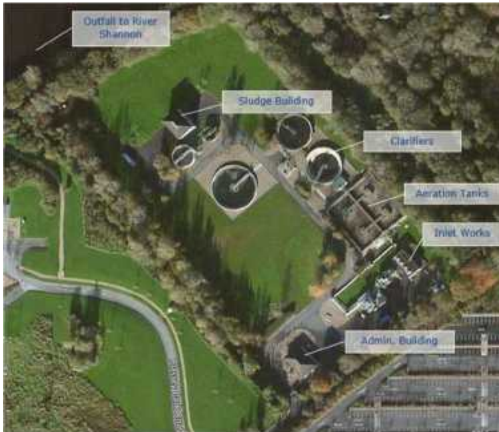
Figure 1.2: Castletroy WwTP Existing Layout
