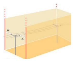
The contractor failed to comply with requirements set out in the "Code of Practice for Avoiding Danger from Overhead Electricity Lines" **to carry out work** in the "Hazard Zone" of Overhead Electricity Lines. See Photo below of the work area in the Hazard Zone of Overhead Electricity Lines:
