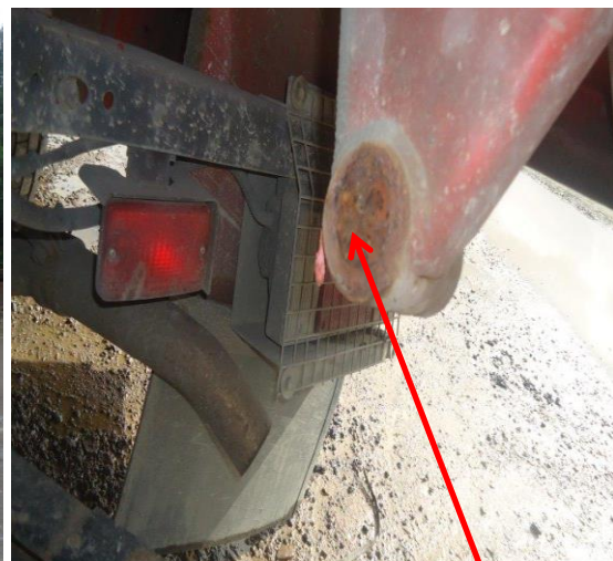
Sheared end of pivot bar seized within bracket
