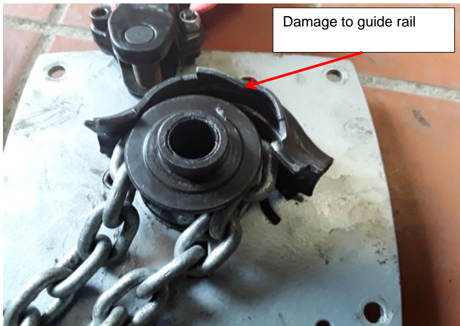
Fig 1 Exposed Incorrectly positioned Chain Guide & damaged guide rail
