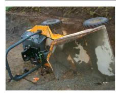
Roll Over Protection System or ROPS are designed and fitted to machinery which on overturning would reduce the possibility of an operator from being crushed, provided the operator was wearing a seat belt. The following points must be taken into account when operating plant with a Roll Over Protection System.
